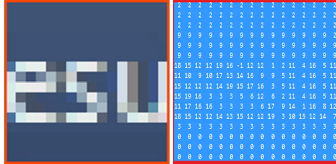
Figure 6.3: Sample PLT Block and Corresponding Index Map
