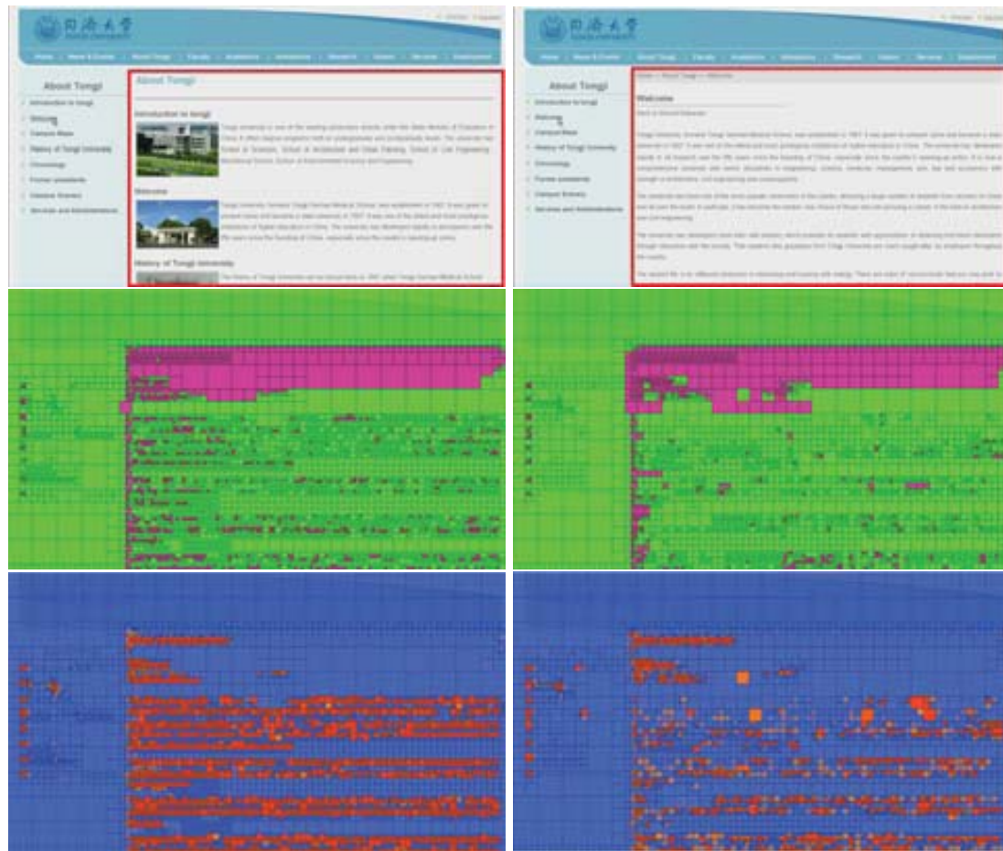
Figure 6.8: Transcoding Analysis of “WebBrowsing” (QP=22). Top Left: 8th Frame; Top Right: 9th Frame; Mid Left: Anchor Transcoding Mode and Partition Decisions; Mid Right: Proposed Transcoding Mode and Partition Decisions; Bottom Left: Anchor Transcoding Bit-Allocation. Bottom Right: Proposed Transcoding Bit-Allocation. Red box: Intra-coded blocks; Green box: Inter-coded blocks; Blue box: low-bit blocks; Orange box: high-bit blocks using color depth to indicate bit-consumption level.
