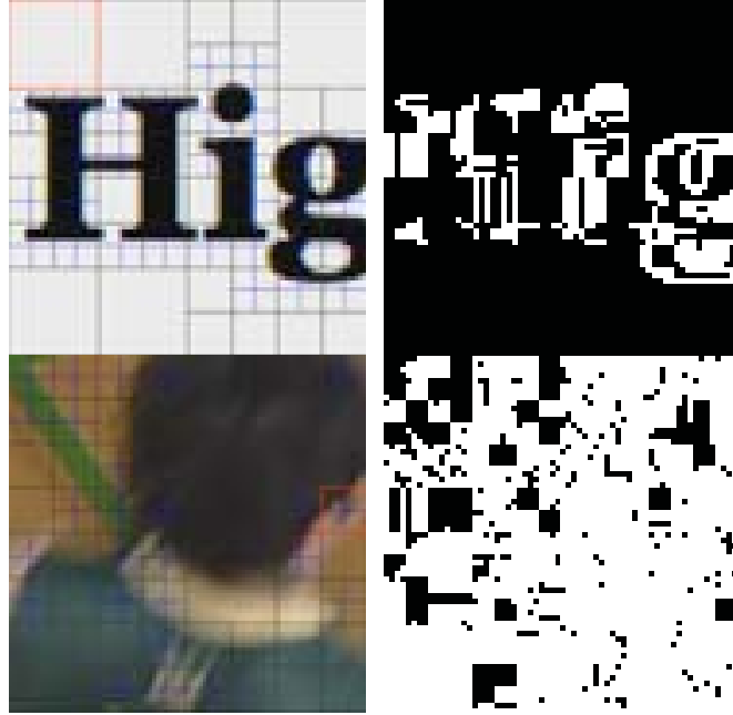
Figure 5.4: SCB and NIB Intra-coding Residual Analysis (Top: SCB sample; Bottom: NIB sample; Left: Image Pattern; Right: Residual Map using white pixels to indicate nonzero entries)
